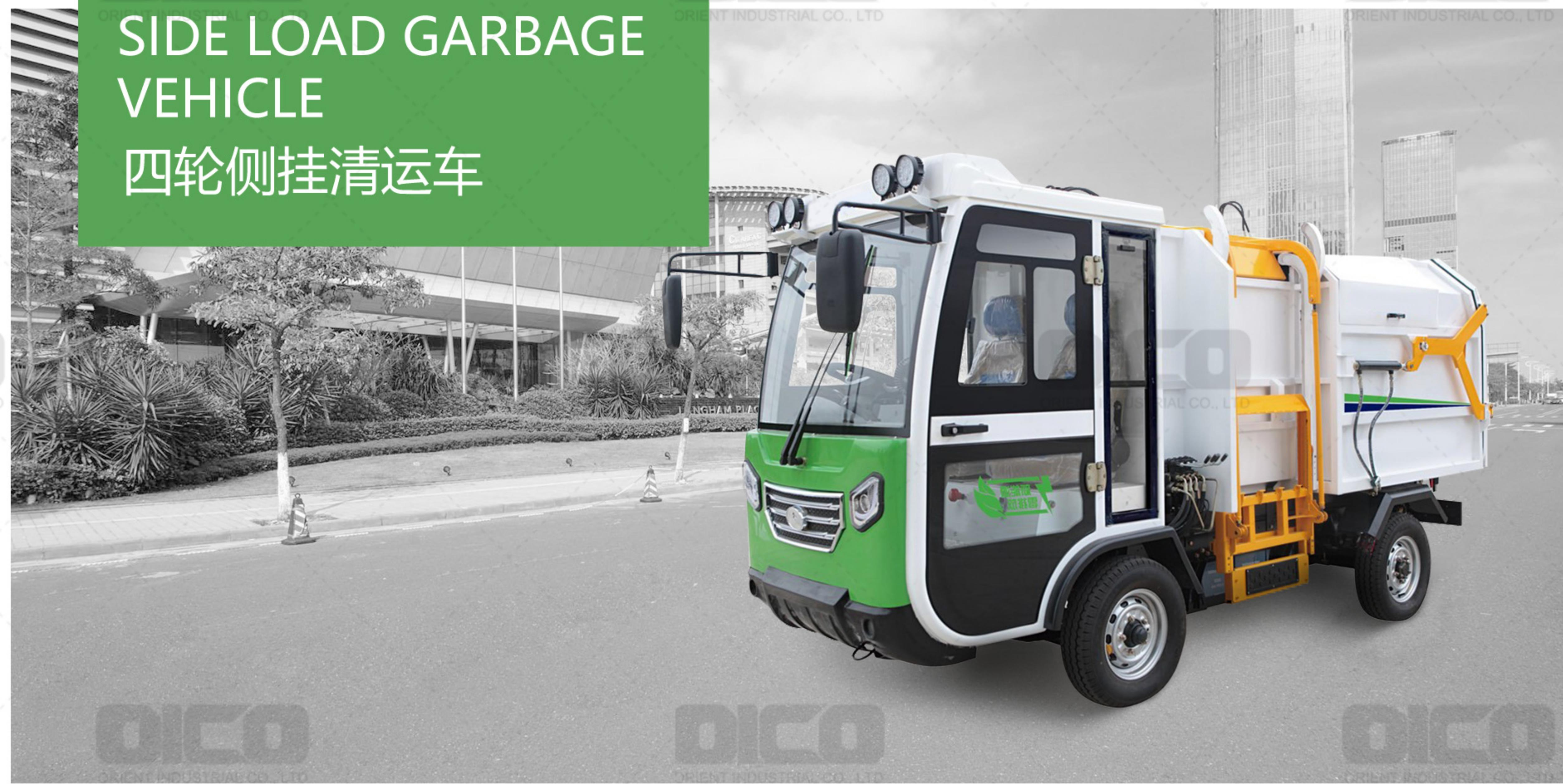
OR-H92 is a side-mounted pure electric garbage collection vehicle, which integrates the dumping device and the garbage dump device. It is suitable for the transportation of garbage in the sanitation and cleaning departments.
